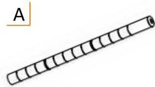
BOTTOM POLE (4) Threaded Insert (4), and Feet Leveler (4) are pre-installed
