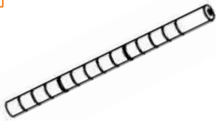
BOTTOM POLE (4) Threaded Insert (4) pre-installed
